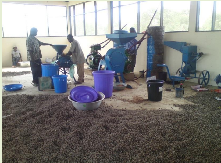
Fig. 3: Processing hall showing some of the processing equipment and sorted shear kernels spread on the floor for aeration before processing.
